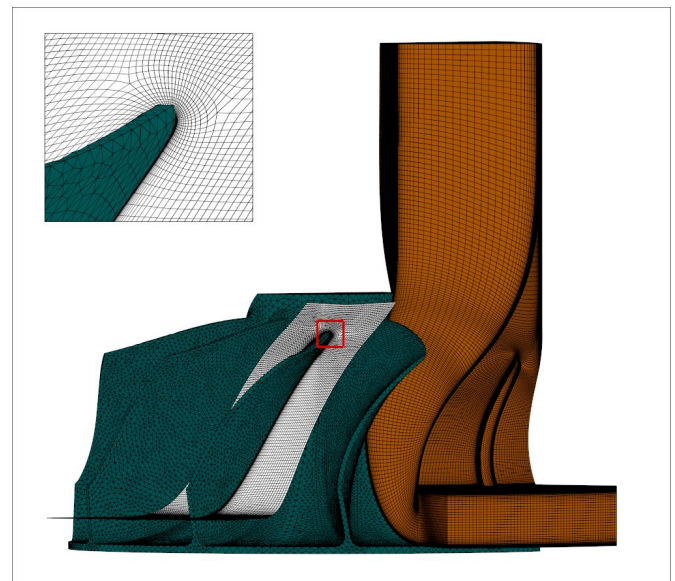
Figure 5 Orange: Structured Grid for Fluid Analysis. Green: Unstructured Grid for Solid Analysis.
